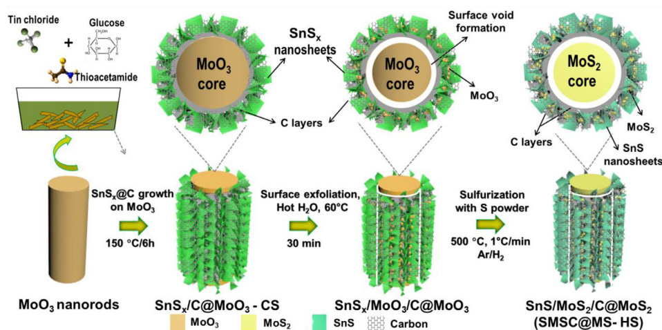
Fig. 1. Schematic presentation for the preparation of SMSC@MS-HS via hydrothermal and eco-friendly surface exfoliation strategy.
